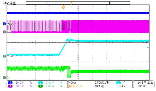
Figure 18. Over Current Release (hard short to 3A)
