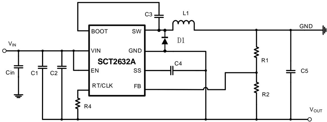
Figure 12. SCT2632A Inverting Power Supply
