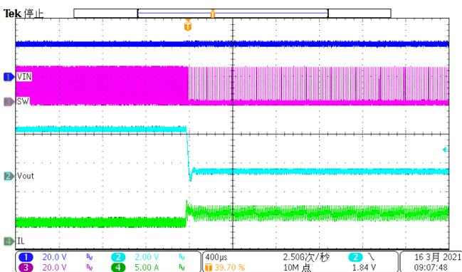
Figure 17. Over Current Protection(3A to hard short)
