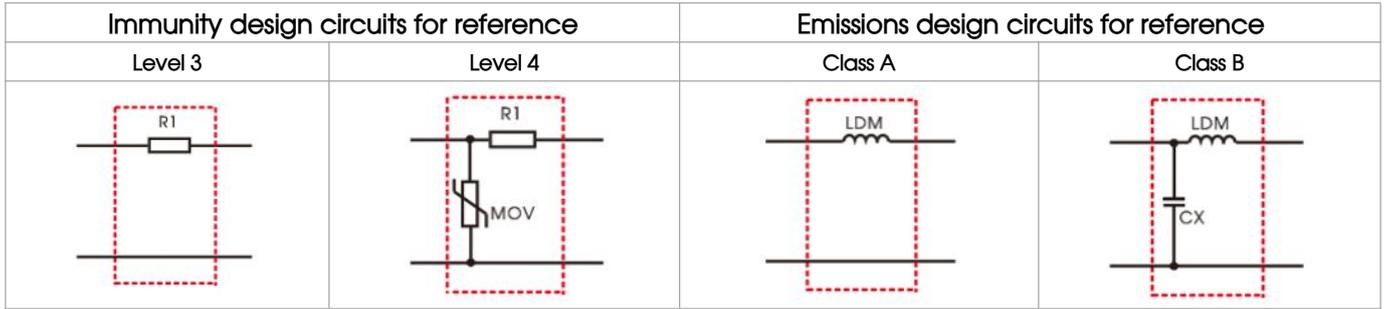
Electromagnetic Compatibility Solution—Recommended Circuit
