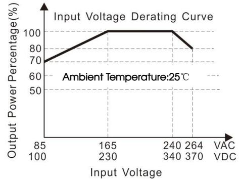
Note: ① With an AC input between 85-165V/240-264VAC and a DC input between 100-230V/340-370VDC, the output power must be derated as per temperature derating curves;
