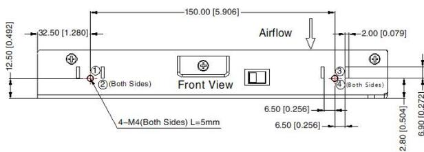
①-⑧ any position must be connected to the earth (⊕)
