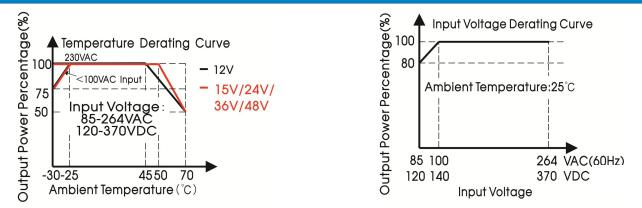
Note: 1. With an AC input voltage between 85 -100VAC and a DC input between 120 -140VDC the output power must be derated as per the temperature derating curves;
