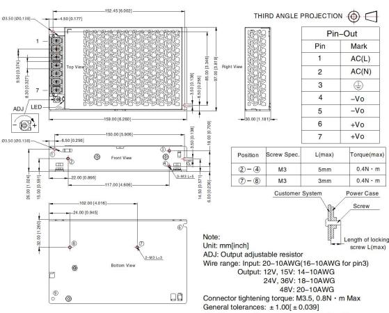
(1-9) any position must be connected to PE
