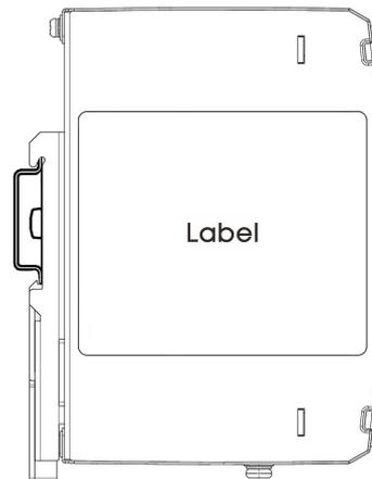
Note: Keep the following installation clearances: 20mm on the top, 20mm on the bottom, 5mm on the left and right sides are recommended when the device is loaded permanently with more than 50% of the rated power. Increase this clearance to 15mm in case the adjacent device is a heat source (e.g. another power supply).
