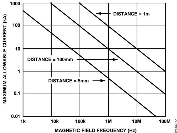
Figure 26. Maximum Allowable Current for Various Current-to-ADuM5200/ADuM5201/ADuM5202 Spacings
