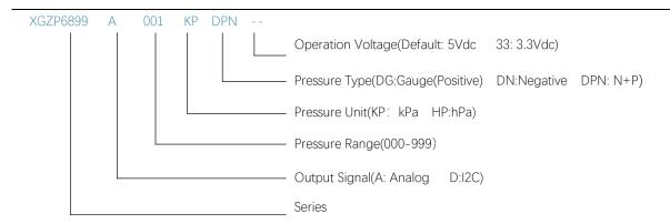
Note: Custom requirement or parameter(e.g pressure range, output etc.,), consult with CFSensor on Part Number.
