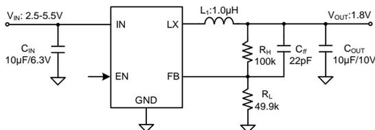
Figure1. Schematic Diagram
