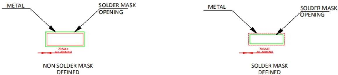
Figure 9.3 SOW8 Package Board Layout Example
