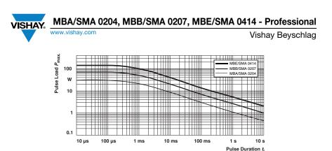
Maximum pulse load, single pulse; for permissible resistance change equivalent to 8000 h operation. Single Pulse
