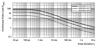
Maximum pulse load, continuous pulses; for permissible resistance change equivalent to 8000 h operation. Continuous Pulse
