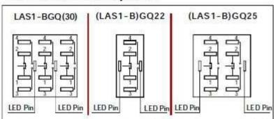
1,2,3,4 are one set;1,2 are normal closed(NC);3,4 are normal opened (NO). The standard LED terminals have no difference of anode and cathode. The lamp and switch are relatively independent and can use switch or peripheral circuit to control the lamp state.
