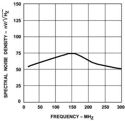
Figure 13. Typical spectral noise density vs. frequency.
