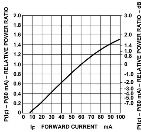
Figure 10. Normalized transmitter output vs. forward current.
