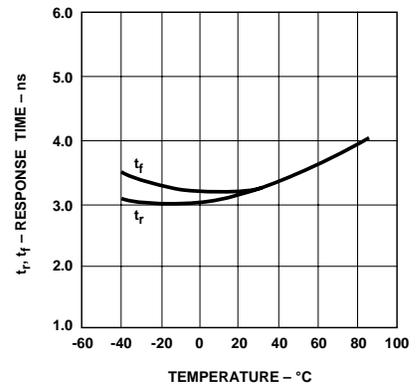
Figure 15. Typical rise and fall times vs. temperature.
