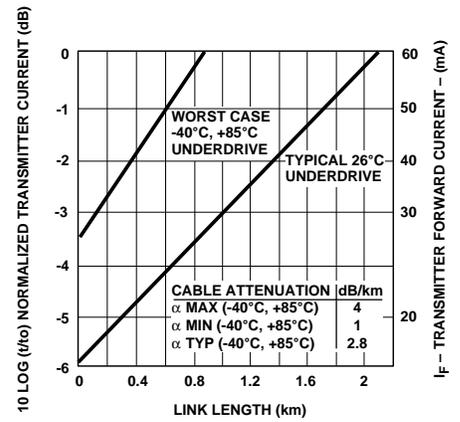
Figure 5. HFBR-14X4/HFBR-24X2 link design limits with 50/125 μm cable.
