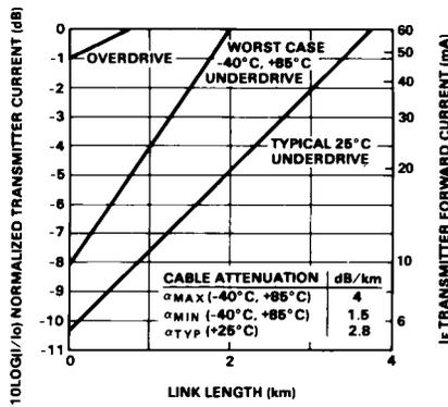
Figure 3. HFBR-1414/HFBR-2412 link design limits with 62.5/125 μm cable.
