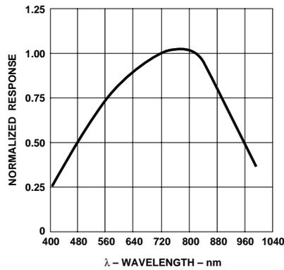
Figure 16. Receiver spectral response normalized to 820 nm.
