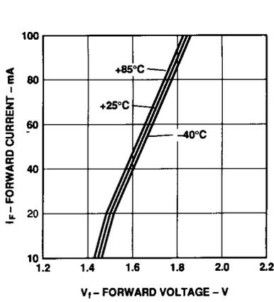
Figure 9. Forward voltage and current characteristics.
