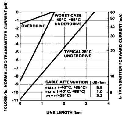
Figure 4. HFBR-14X2/HFBR-24X2 link design limits with 100/140 μm cable.
