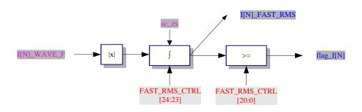
7 channels have fast effective value registers, which can detect half cycle or cycle effective value. This function can be used for overcurrent detection.
