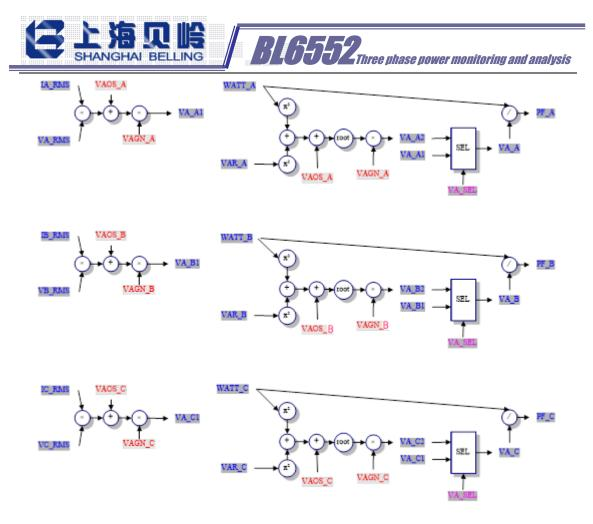
There are two ways of apparent calculation: One is the digital multiplication of the effective value of the current and voltage, and then the apparent power signal can be obtained after gain and offset calibration. The active power is divided by the apparent power to obtain the power factor.
