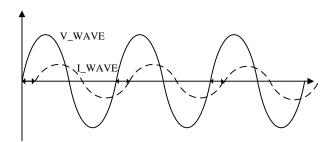
The phase difference is obtained by calculating the time difference between the positive phase zero crossing of the current and the voltage, and the corresponding time value is updated to the register CORNER[N]. Each register is a 16-bit unsigned number.
