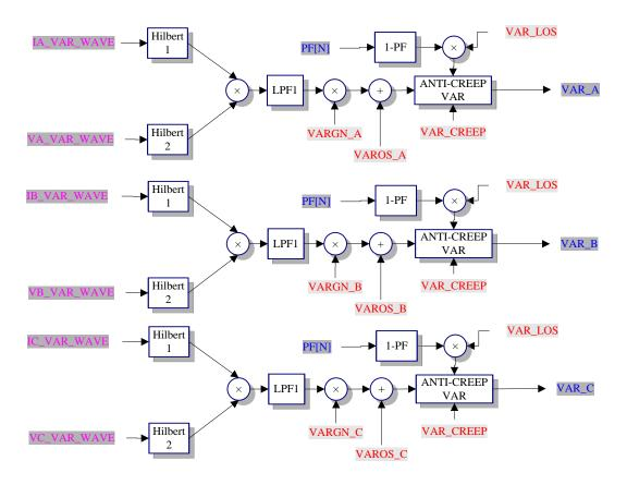
After the current and voltage waveforms of each phase pass through the Hilbert filter, digital multiplication is performed, and then the reactive power signal can be obtained after the low-pass filter, gain and deviation calibration, anti-creeping judgment and averaging processing in order. After integration, the reactive energy pulse accumulation is obtained.
