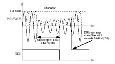
As shown in the figure above, when the instantaneous effective value of the voltage is less than the threshold set in the drop voltage threshold register (SAGLVL) and the drop time exceeds the set time in the drop line period register (SAGCYC) (the figure shows after the sixth half cycle is exceeded, SAGCYC[11:0]=06H), the line voltage drop event is recorded by setting the SAG flag bit in the interrupt status
