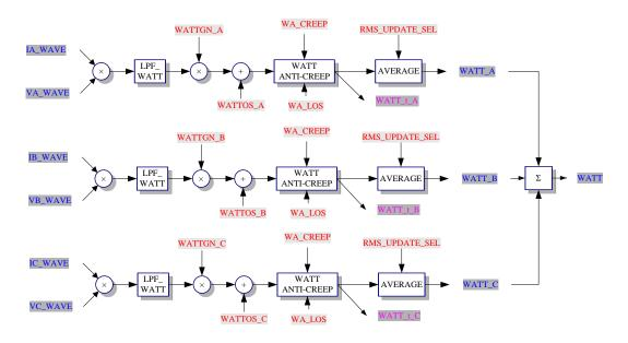
The three-phase current and voltage waveforms are respectively digitally multiplied, and then passed through the low-pass filter, gain and deviation calibration, anti-creeping judgment and averaging in order to obtain the split-phase power signal, which is added to obtain the total active power.
