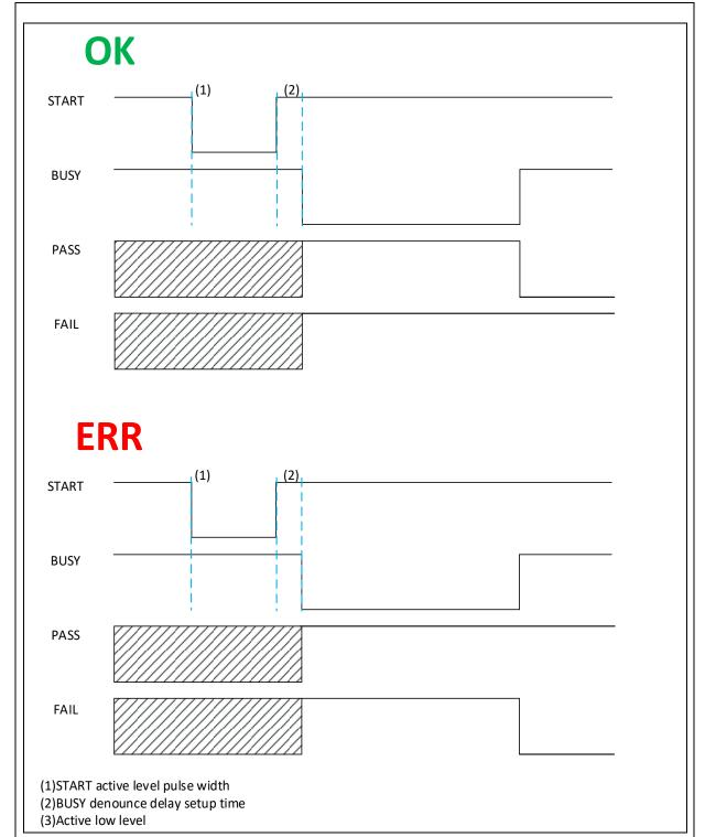
Figure 30. Typical timing diagram of machine programming control
