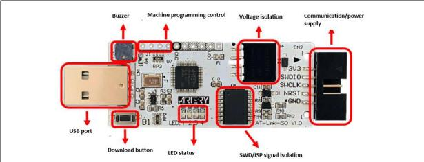
Figure 4. AT-Link-ISO hardware appearance
