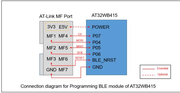
Figure 6. MULTI FUNC interface connected to AT32WB415 BLE module
