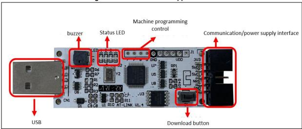
Figure 1. AT-Link hardware appearance
